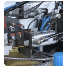
Replacement of pneumatic cylinders
